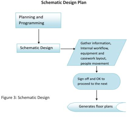
In a laboratory project it is beneficial to show all major equipment, whether countertop or floor mounted in the schematic design. This assists in the discussion of specific workflows and staff movements. It also illustrates whether sufficient workspace is allowed for each instrument and procedure.
